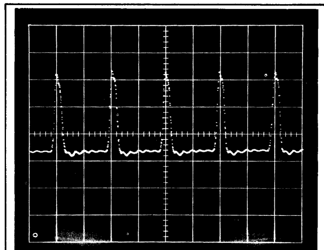
(A) 2 div between markers with VARIABLE control at CAL (detent) position.
